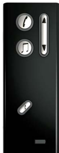
Streamer - Uses a wireless Bluetooth connection to connect Agil to electronic instruments such as phones, TV, MP3 players and more.
