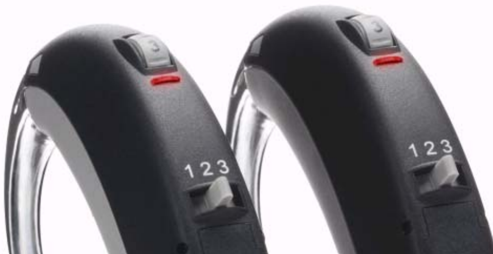
Figure 2. Oticon Sumo volume control wheel and alerting LED.
