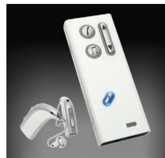
Figure 1: A body-worn gateway device that transmits audio signals to a pair of hearing aids using digital magnetic transmission.
