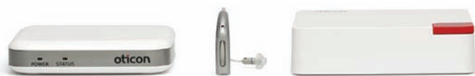
Figure 2: Adaptors designed to send landline phone (right) and television (left) audio signals to a gateway device.
