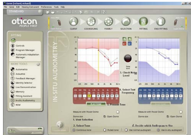
Figure 2: In-situ test screen with recommended steps for testing added (above) to serve as a quick guide to ensure the parameters are set correctly for in-situ testing.
