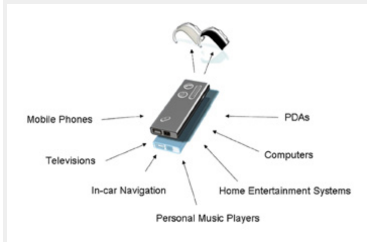
FIGURE 1. Examples of far-world signals the Oticon Epoq Streamer can transmit to the Epoq hearing instruments.
