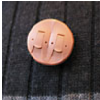
Figure 1. The original Syncro datalogger used in verification studies of advanced hearing instrument systems. Note the two sets of directional microphone inlets so that the impact of two sound processing strategies could be measured simultaneously.
