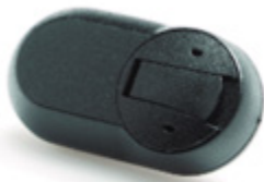
FIGURE 1. The Sound Activity Meter (SAM), a commercially usable, client-worn envirometer (about 3/4-inch in length).
